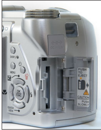
FIGURE 5.29 Pay attention to the doors and covers a camera uses for its media, batteries, and ports. You'll be opening and closing these a lot, so make sure they're sturdy and durable.
